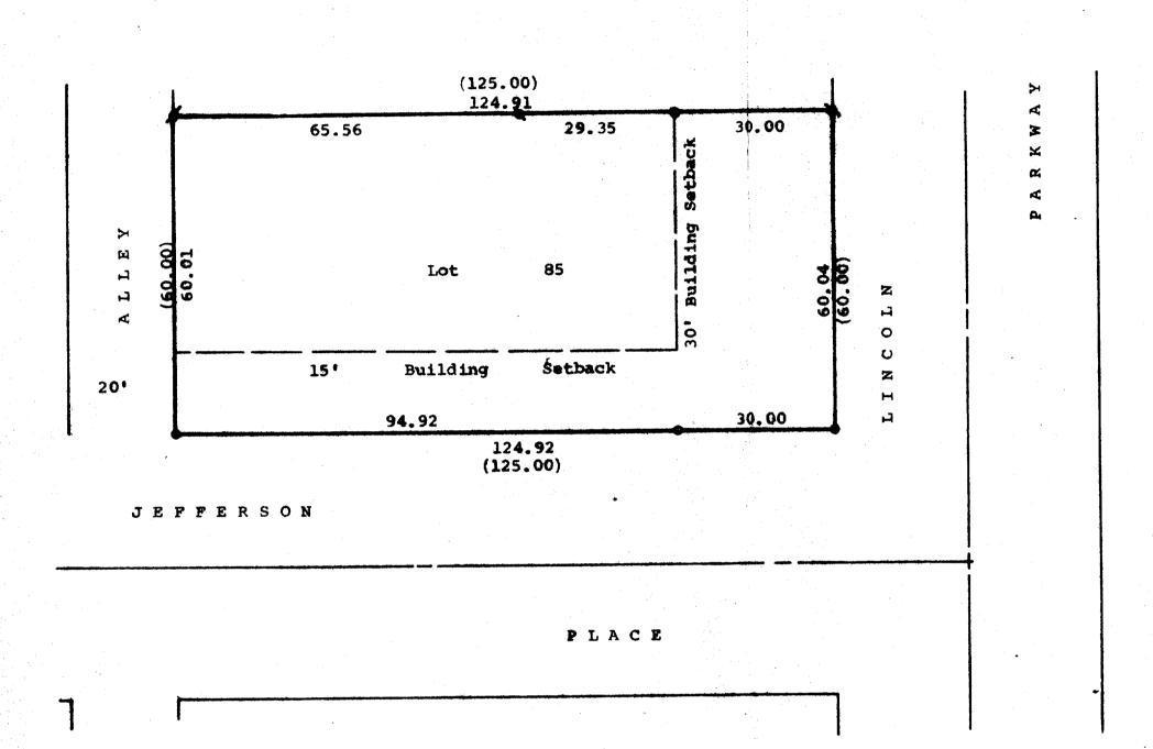
Scale - 1" = 20' • = Concrete Monument a - Iron Pipe Found #= Iron Rod Found o = Iron Pipe Set (0.00) = Recorded As
